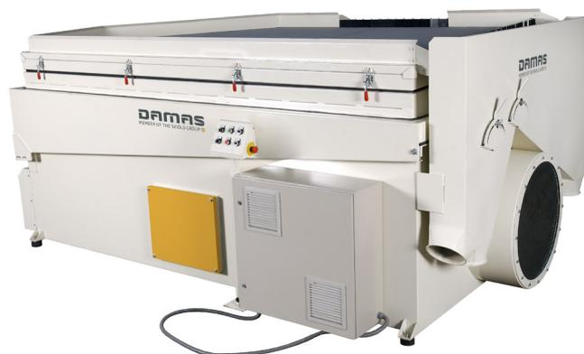
The ZETA is available with half or full dust hood and recirculation and with several deck types for different products.
